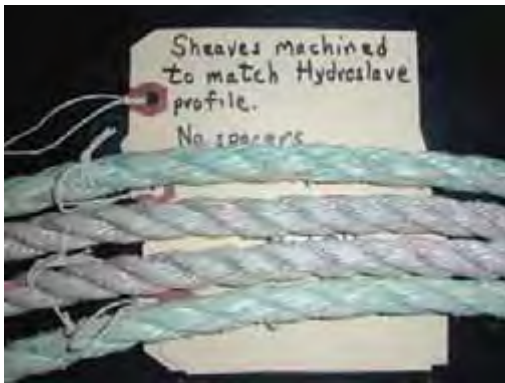
Figure 18. Rope samples from Treatment 19, sheaves machined to match Hydroslove variable surface angle stamped steel sheaves. The aqua colored rope is Polysteel © floating rope and the gray rope is a blended polyester and Polysteel © sinking rope.
