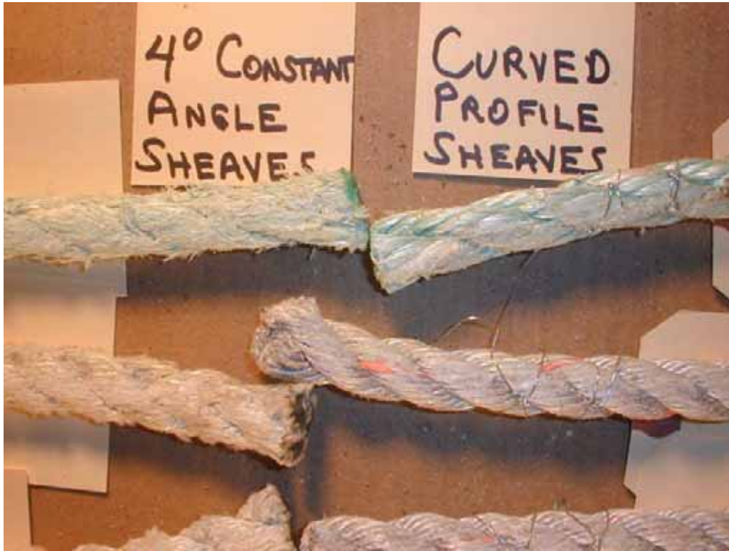
Figure 32. The standard 4-degree constant angle offshore sheaves cause more damage to the rope fibers than can be seen on ropes run on variable angle sheaves.
