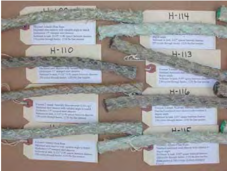
Figure 20. The four samples on the left are from Treatment 19, the variable angle machined sheaves. The samples on the right are from the standard, constant 4-degree angle machined sheaves. The samples on the left have a higher residual breaking strength that is statistically significant. Contrary to appearances, the breaking strength of the floating Polysteel © (light green) samples is higher than the residual breaking strength of the blended polyester/Polysteel © sinking rope.
