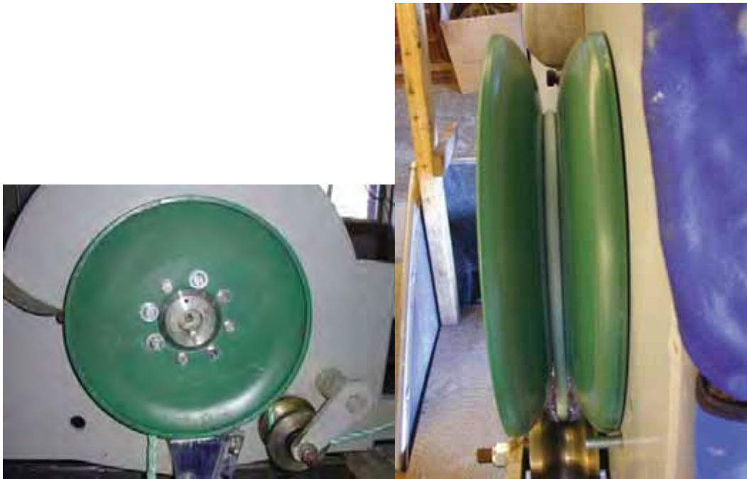
Figure 15. Front and side views of 17-inch Hydroslove stamped steel hauler sheaves that showed the least rope wear of any of our hauler treatments.
