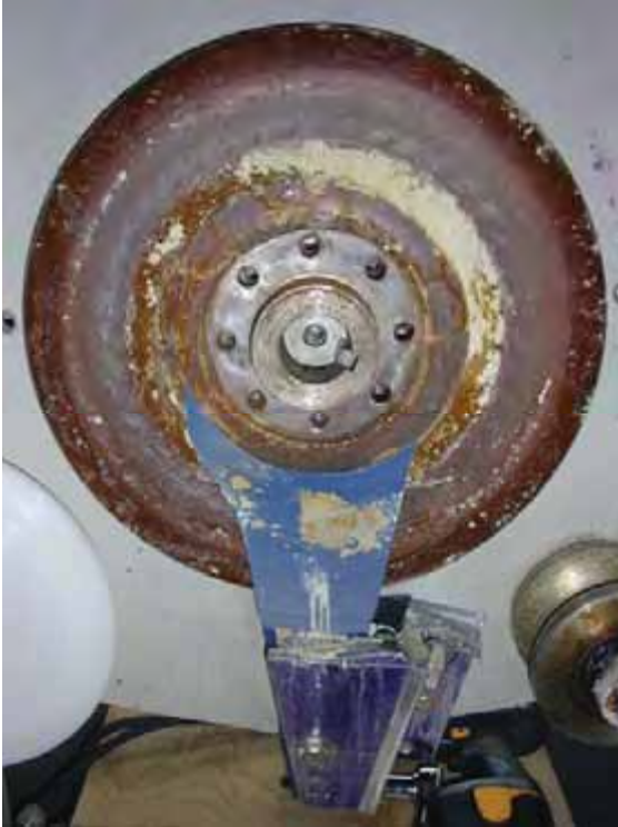
Figure 16. Treatment 11 utilized a low angle of incidence splitter machined from ultra-high molecular weight polyethylene.
