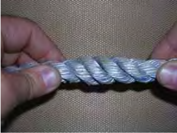
Figure 9. Our observations indicated that the standard splitter can cause rope “bunching” similar to that seen in this picture under certain conditions. Bunching of the rope makes it more likely that a strand of rope will jam between the splitter and the sheaves.
