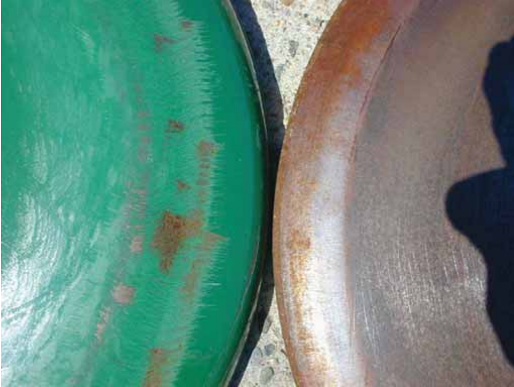
Figure 12. Slightly used Hydroslave 17" stamped steel sheaves next to machined steel sheaves. Hydroslave sheaves begin life with a smooth painted finish, which has been scuffed up in the picture above. Machined steel sheaves begin life with circumferential ridges left by the tooling. The depth and spacing of the machining ridges varies from machine shop to machine shop, and can be specified by the customer.
