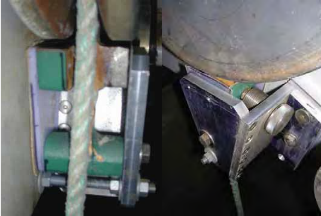
Figure 23. The picture on the left shows the rope being guided out of the hauler sheaves by the splitter. The picture on the right shows the load cell mounted behind the splitter on the hauling simulator. The knife was allowed to pivot on one bolt, exerting pressure against the load cell.
