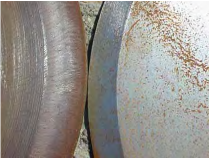
Figure 13. Two sets of machined steel sheaves showing differences in the circumferential ridges left by the lathe.
