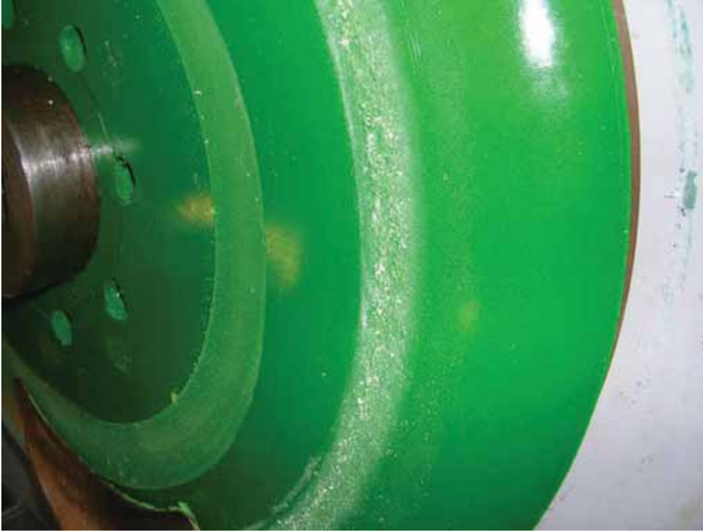
Figure 17. 47 Shore D polyurethane sheaves showed excessive wear after a short period of simulated hauling.
