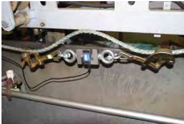
Figure 5. Computer connected electronic load cell attached to groundline on simulator to measure in-line tension in rope running on the simulator.
