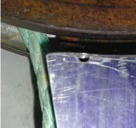
Figure 24. This picture shows clearly how the Polysteel © rope cleared the variable angle sheaves with no spacing without contacting the splitter within the radius of the sheaves.
