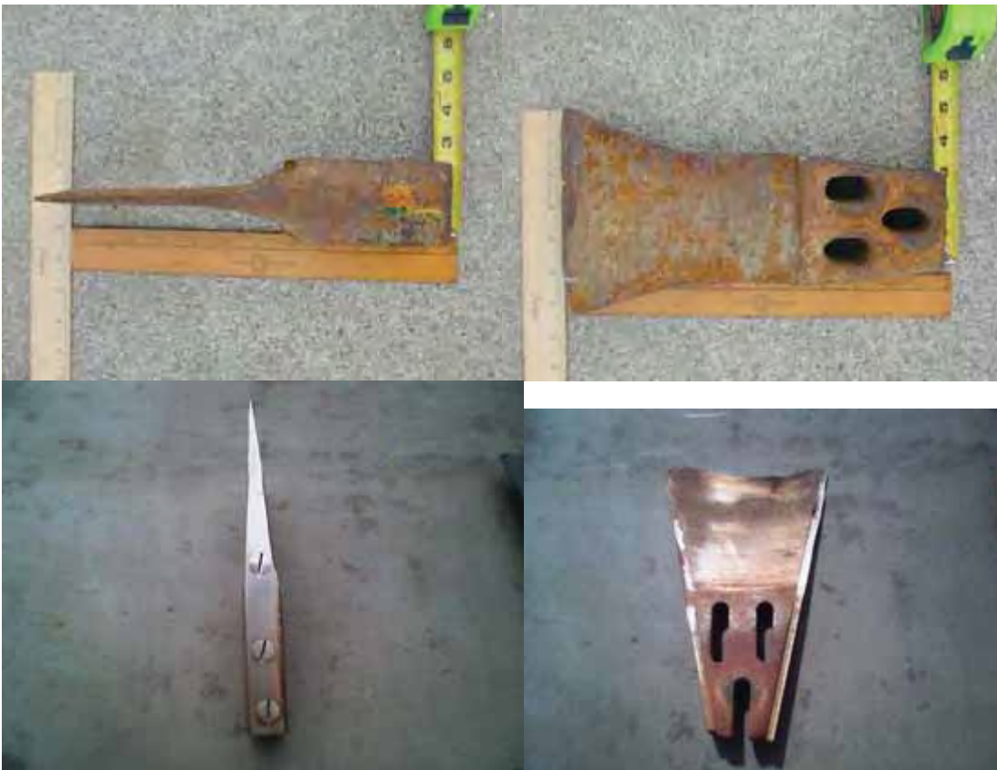
Figure 25. Steel wedges force ropes out of the v-groove between the hauler sheaves so that the rope won't simply wind around the hauler. These rope extractors (commonly referred to as splitters or knives) are made in a variety of shapes. Splitters tend to wear rapidly, forming a groove with sharp edges. The splitter in the bottom half of this picture has a replaceable stainless steel wear plate. The condition and fitting of the splitter are critical to rope longevity.
