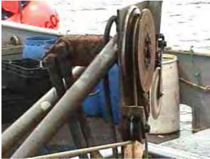
Figure 1. Trap hauler on offshore lobster boat showing rope leading into hauler through fairlead block. Disc at the bottom right of hauler exerts pressure on rope to prevent it from jumping out of hauler and is called a “pizza cutter.”
