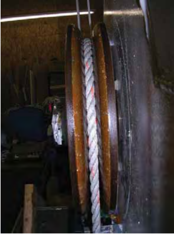
Figure 19. Variable surface angle machined steel sheaves that match the surface profile of Hydroslave stamped steel sheaves. With no spacer between the sheaves, the rope rides close to the outer rim where the angle between the sheaves is widening beyond the 4-degree angle of the standard offshore sheaves.
