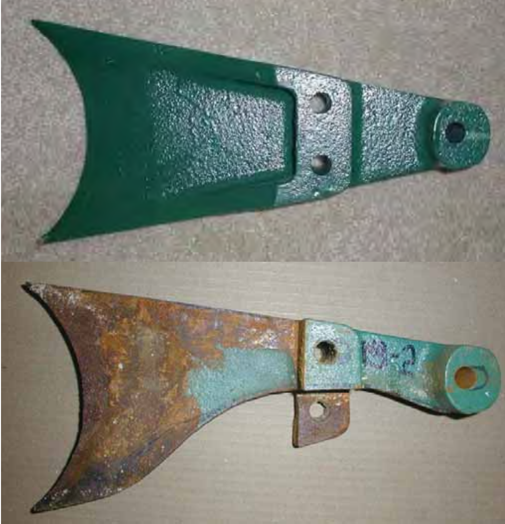
Figure 10. Comparison of standard cast steel Hydroslove rope splitter (top) with modified splitter that incorporates a reverse curve for the purpose of reducing the angle at which the rope impinges on the splitter.
