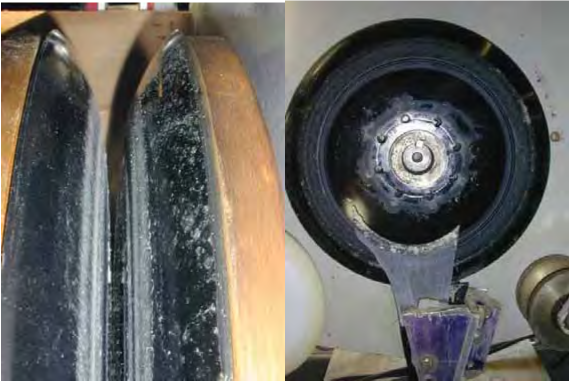
Figure 22. Images of harder durometer (65 Shore D) polyurethane sheaves after 14 hours of simulated hauling. Treatment 19 also utilized a splitter molded with 65 Shore D polyurethane.
