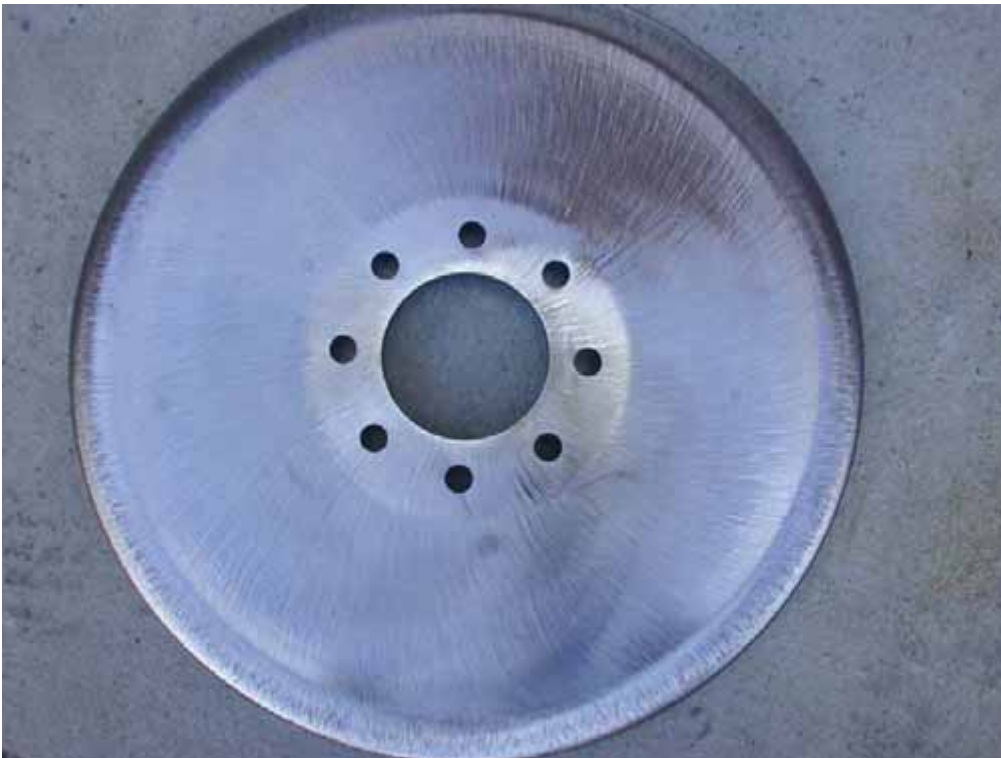
Figure 21. Newly machined sheaves that have been finished with a rotary grinder show the vestiges of circular machining ridges as well as the radial marks of the grinder. These surface irregularities contrast with the smooth surface of Hydroslove stamped steel sheaves that showed the best performance in terms of reduced rope wear.
