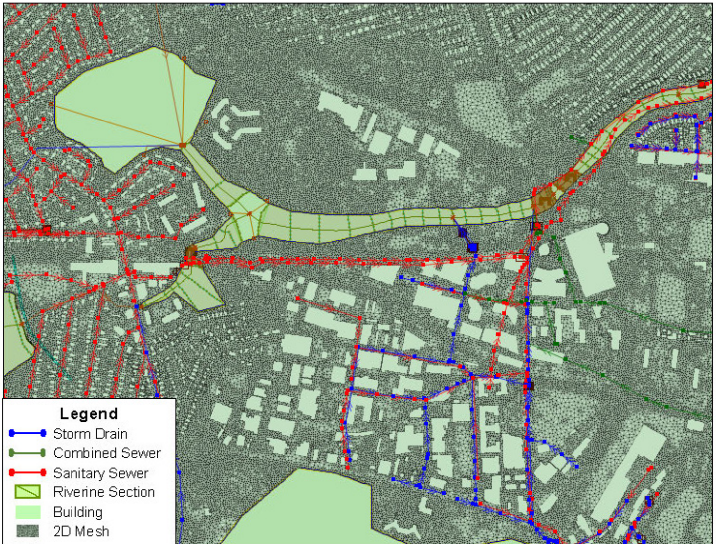
Figure 5 – Example of Interactions Between Surface Mesh, Building Footprints, and Waterways
