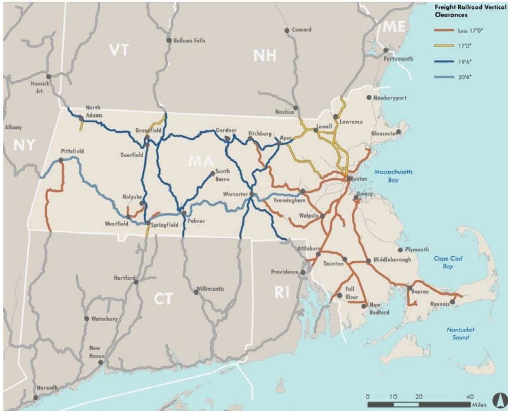
Figure 2-5: Freight Rail Vertical Clearances
