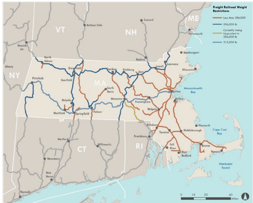
Figure 5-4: Freight Railroad Weight Restrictions
