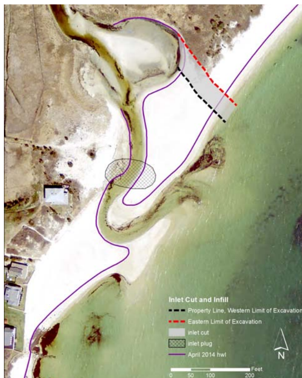
Figure 4: Aerial view of the Meadow Shores Marsh existing inlet and approximate locations of proposed repositioned inlet channel and sand-fill plug in existing channel
