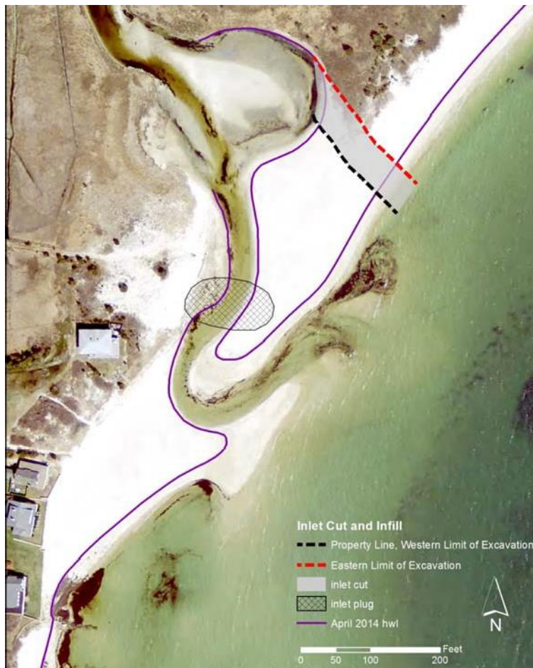
Figure 4: Aerial view of the Meadow Shores Marsh existing inlet and approximate locations of proposed repositioned inlet channel and sand-fill plug in existing channel
