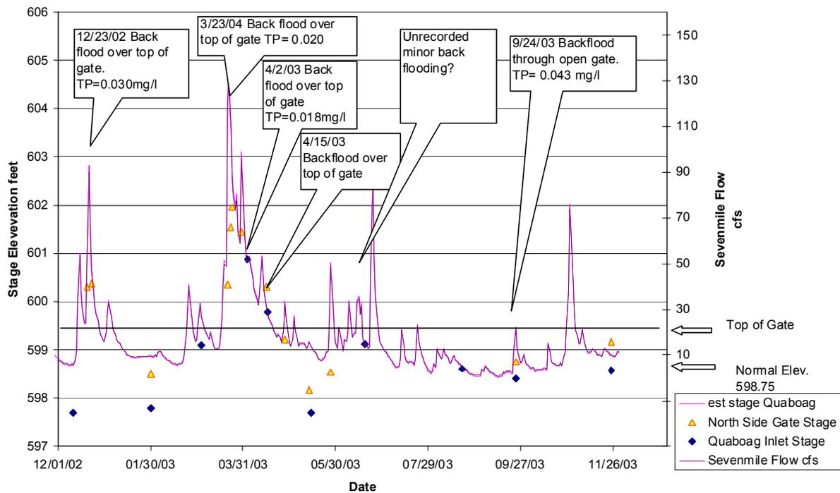
**Figure 13. Water Stage at Quaboag Pond and at Quacumquasit gate.** Water stage level shown as points. The line represents the instantaneous flow rate at the USGS gage on the Sevenmile River at Cooney Road.
