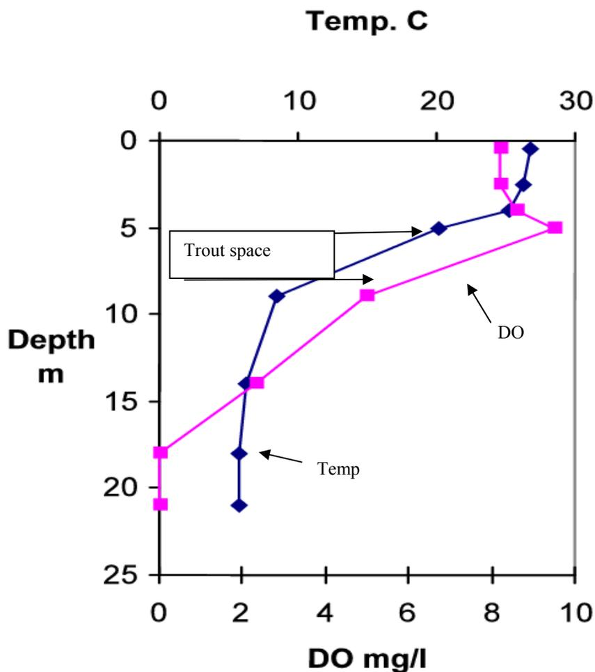
Figure 10. Quacumquasit Pond DO and Temperature 8/20/03.
