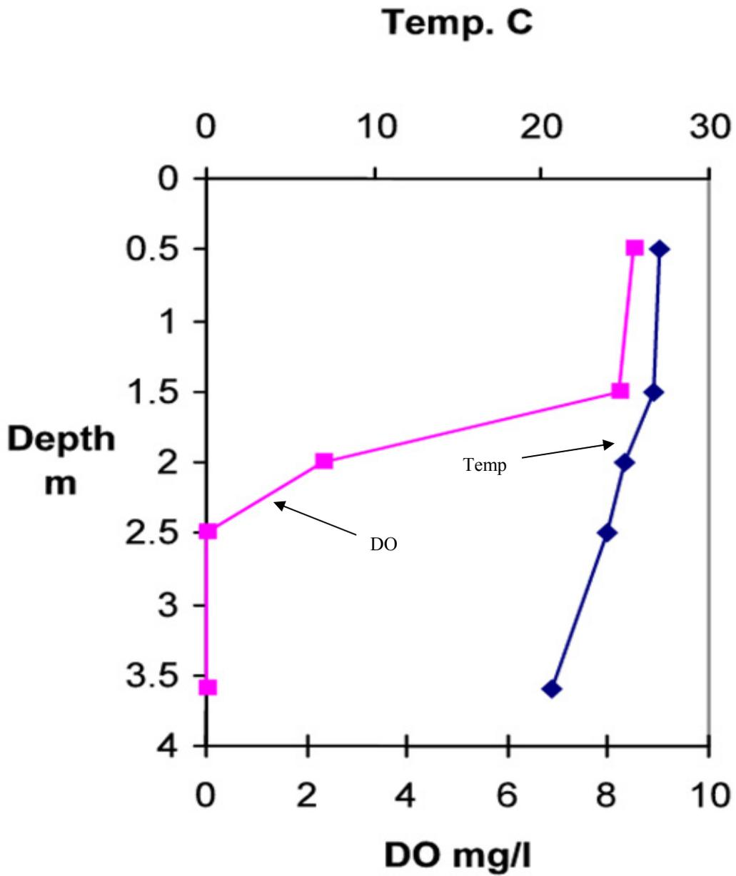
Figure 4. Quaboag Pond DO and Temperature 8/20/03.
