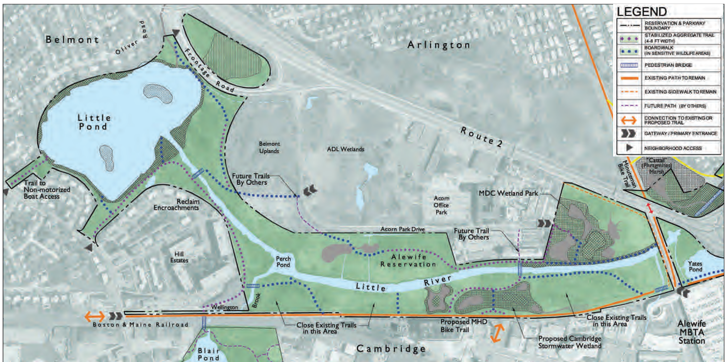
Figure 32: Proposed circulation in Alewife Reservation. The proposed circulation system retains some of the routes of existing trails but converts them to boardwalks to protect sensitive wildlife areas and keep visitors from venturing off the path. Most of the informal trails south of the Little River will be closed using extensive native plantings (thorny species). The proposed paths and boardwalks allow for loop walks, especially in the East Reservation where educational features will enable the area to serve as an outdoor classroom.
