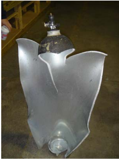
Figure 1. Ruptured Oxygen Cylinder from 2004 Lake Mishnock, RI Fire
