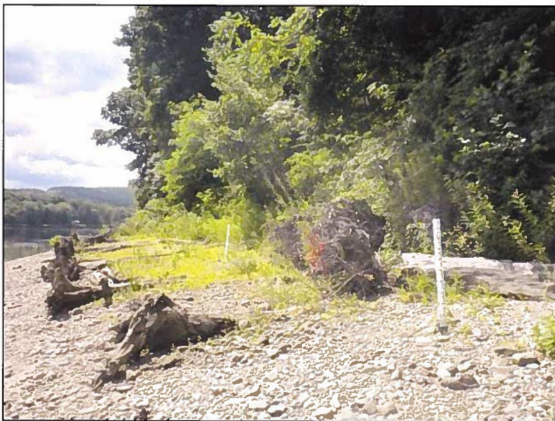
Bathory/Gallagher site: Gauges indicate negative to minimal sediment accumulation
