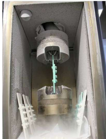
Phase II Mechanical & thermal preconditioning of sealant test vehicles
