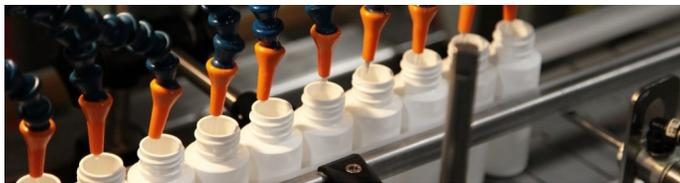
The new pressure gravity filler purchased by US Pack with TURI funds helps to reduce the use of acetone, ethylene glycol and methanol used in manufacturing automotive, industrial and household cleaning products.
