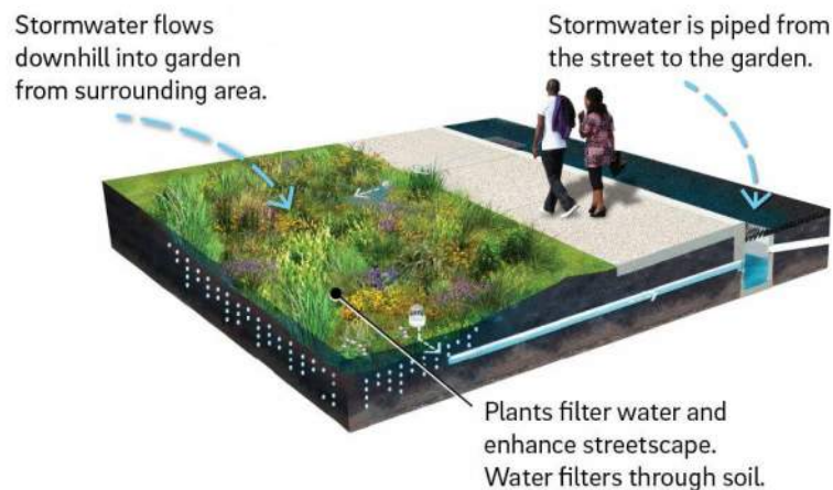
Figure 6-4: Schematic of Bioretention Managing Roadway Runoff
