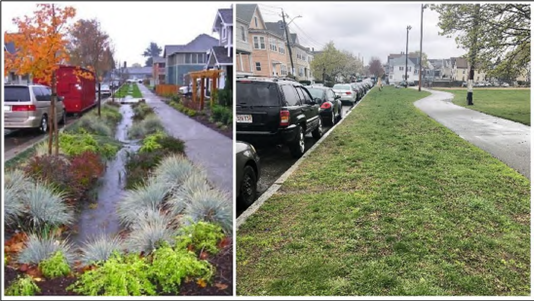
Concept for proposed linear open vegetated swale BMP (refer to detail, Sheet GC-3) (left image source: Biocycle)
