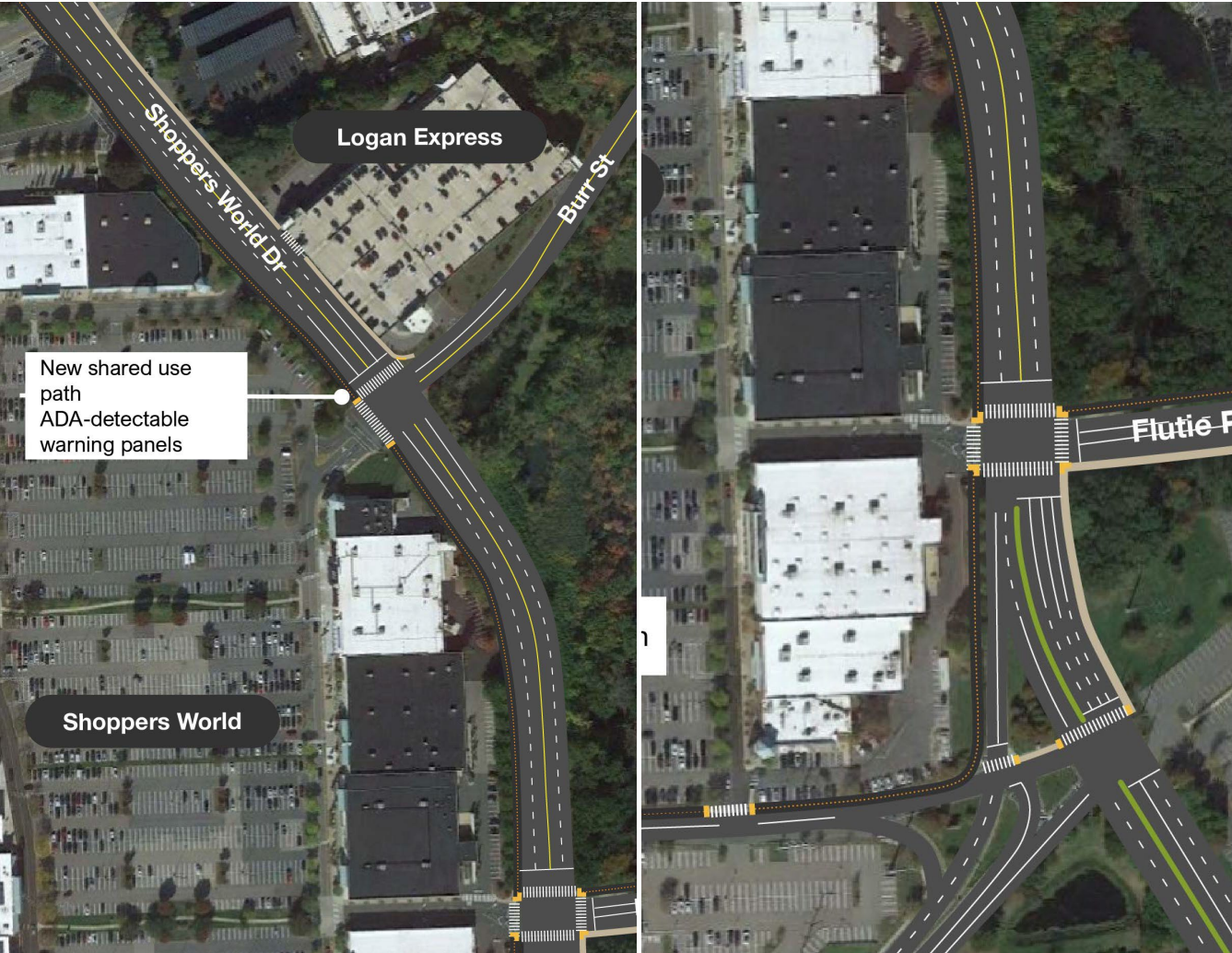
The Proposed Shared Use along Shoppers World Drive connecting Route 30 to Route 9, and creating a protected and dedicated bicycle and pedestrian facility which does not exist today.
