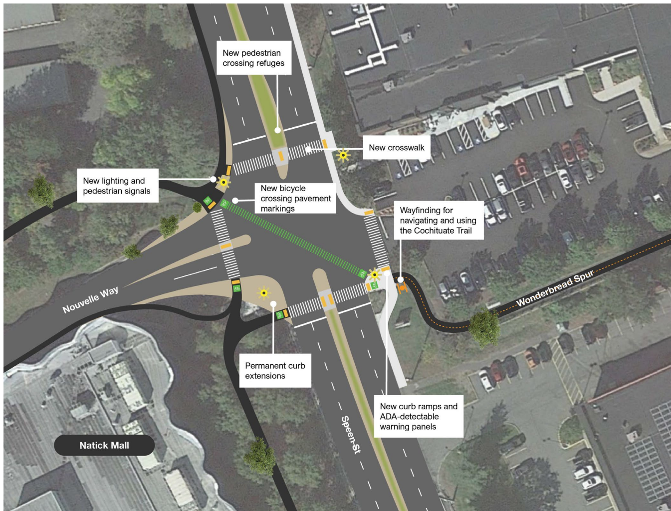
The Proposed Improvements to create a safe and pedestrian/cyclist-oriented intersection at Speen Street and Nouvelle Way.
