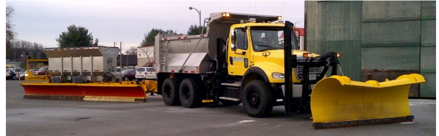
MassDOT dump truck with tow plow equipped for snow and ice
