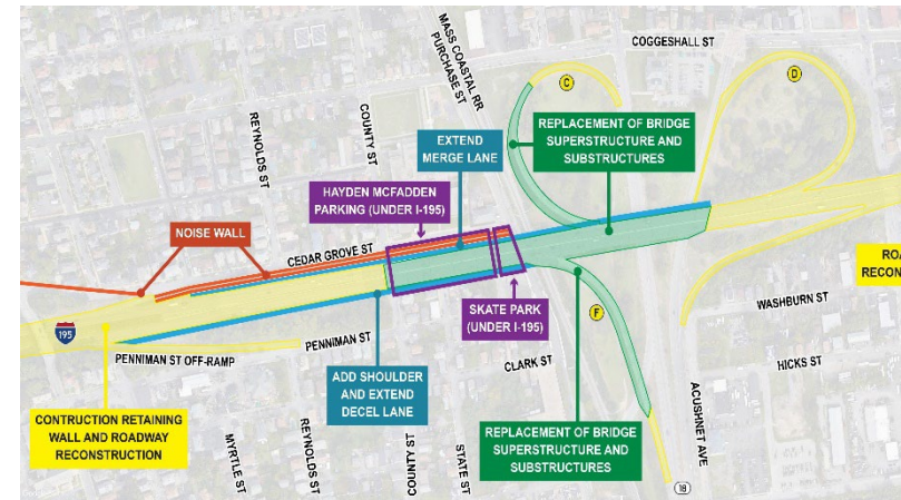
Map of the I-195 to Route 18 Interchange Rehabilitation project in New Bedford
