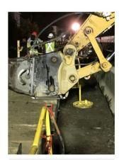
Rock grinder on crane mat; post-incident
