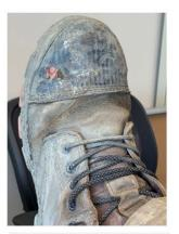
EE's boot with rock grinder contact marks
