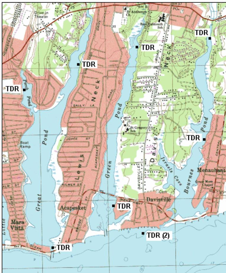
Figure V-12. Map of the study region identifying locations of the tide gauges used to measure water level variations throughout the system. Nine (9) gauges were deployed for one month between January and February, 1999. Each black square represents the approximate locations of the tide gauges.
