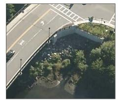
Scour at stormwater outfall to Merrimack River near Bates Bridge.
