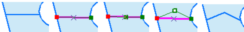
Example of modifying a line and polygon by adding a vertex to edge and dragging it.
