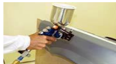
Example of a High Volume, Low Pressure (HVLP) spray gun.
