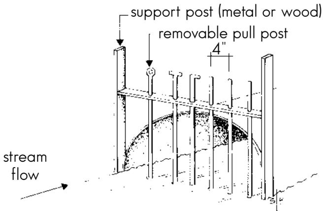
Removable pull rod grill is easier to remove than wire mesh because there are no horizontal bars to catch deposited material. After most material is cleared, posts can be pulled out, allowing the current to wash away any remaining material.
