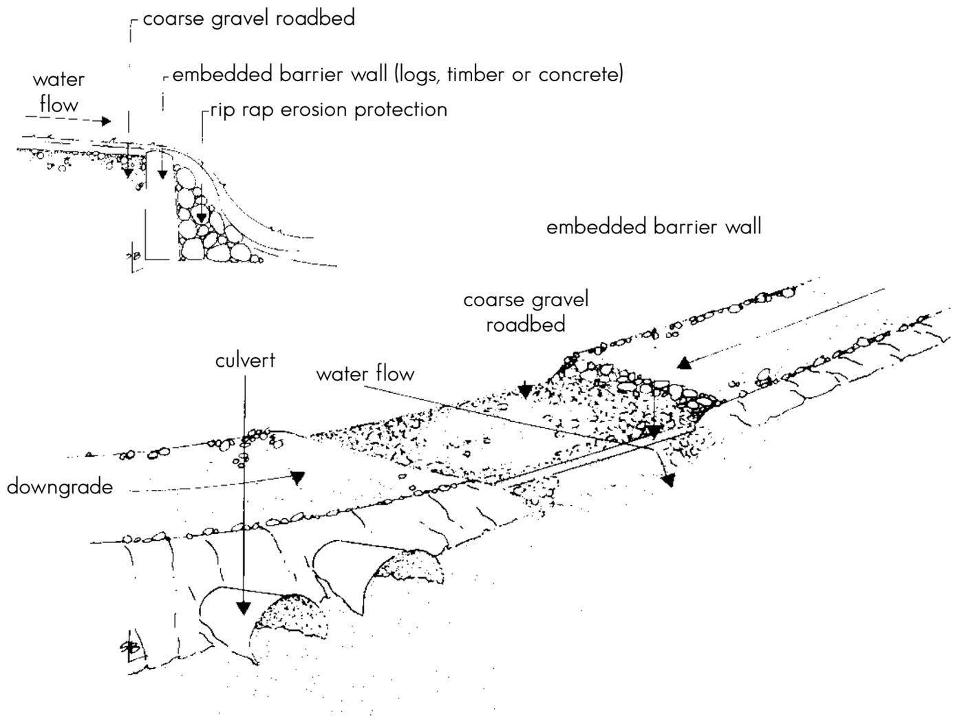
**Low water crossing** If we can accept the fact that a road will experience periodic flooding, then the road can be designed to receive the flowing water with minimal or no damage.
