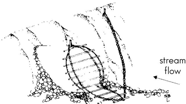
**Culvert protector-cleaner** Constructed by welding steel rods (4 inches apart) across a looped chain: upper end is held by a bolt placed through the top of the culvert; tail end is looped back and anchored on road bank; end of chain can then be attached to a vehicle and the grill flipped up onto the road to clear culvert
