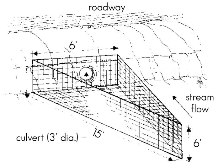
**Triangular screen mesh design** Constructed from 2" mesh welded wire; placed on upstream end of culvert; should be removed during winter to prevent ice damage. Dimensions shown are for a 1 meter culvert, increase measurements if required. (Drawing not to scale).
