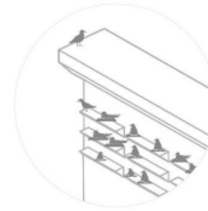
1. Storm wall with ledges for cliff-nesting birds
