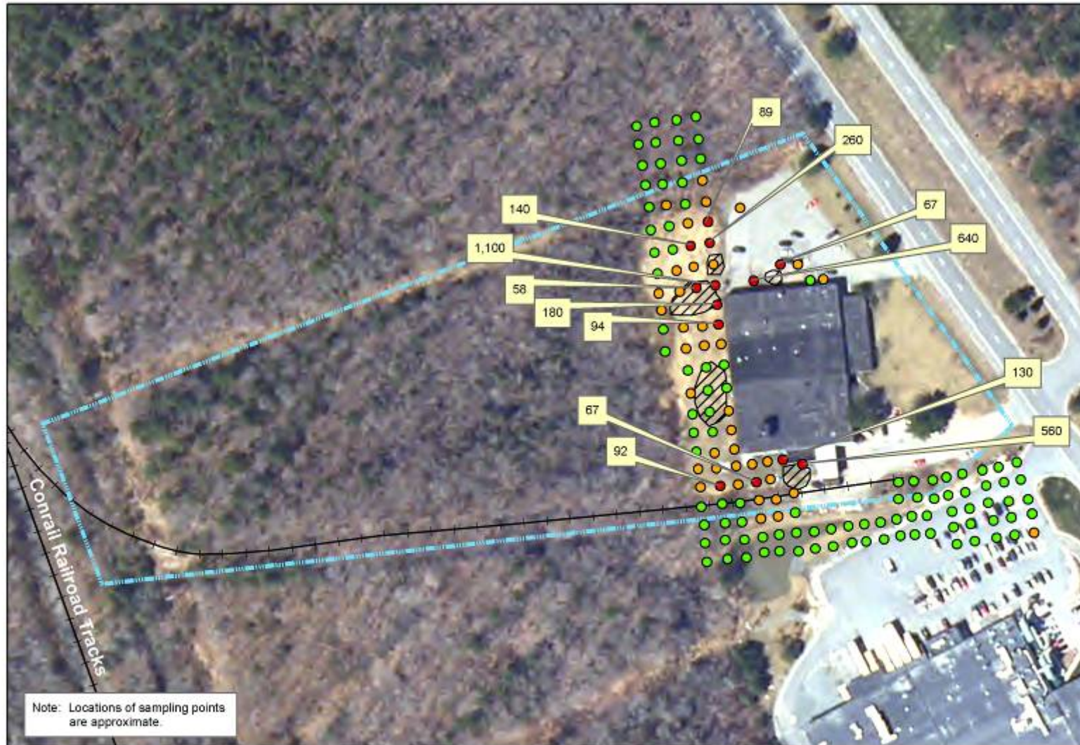
Figure 4 Surface Soil Samples Prior to 2000-2001 Excavation at the Former Polymerine Site New Bedford, Massachusetts
