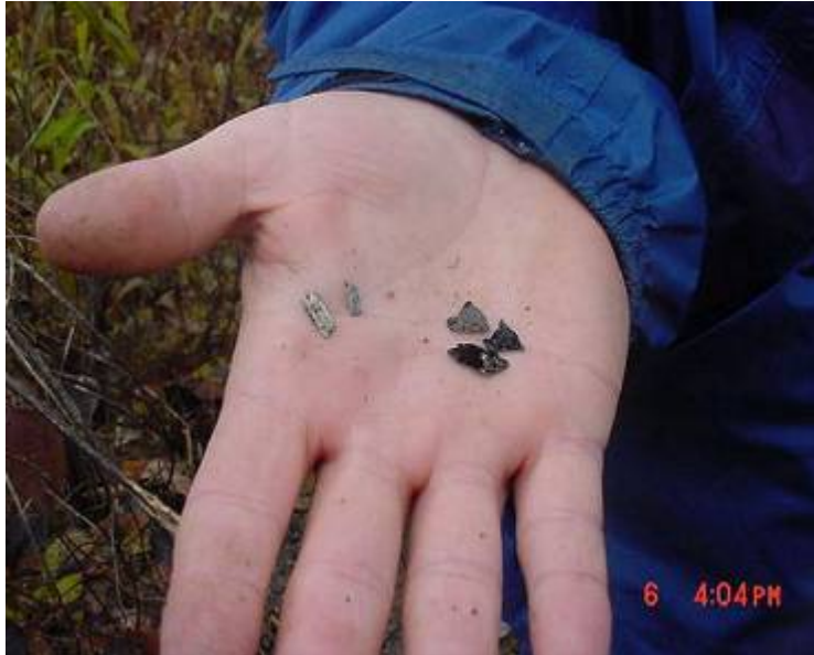
8. Rod-like fibrous asbestos (left) and very shiny, plate-like vermiculite from mound
