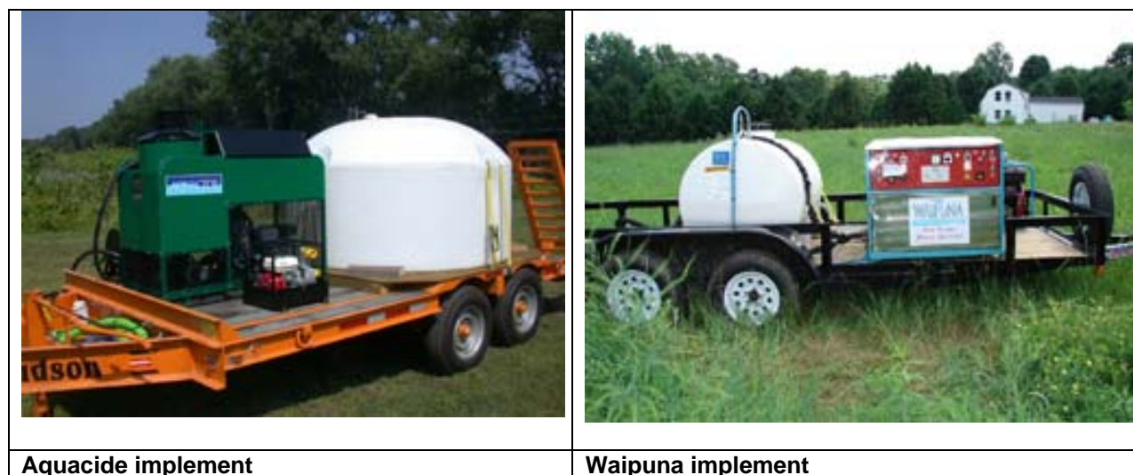
Figure 4.28. Steam application equipment used in research.
