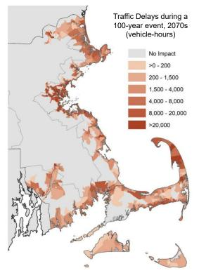
Figure 3.5: Traffic delays impacting emergency response by block group for a 100-year return period coastal flood (one-percent chance of occurring annually) by 2070. (Source 2022 MA Climate Assessment.)
