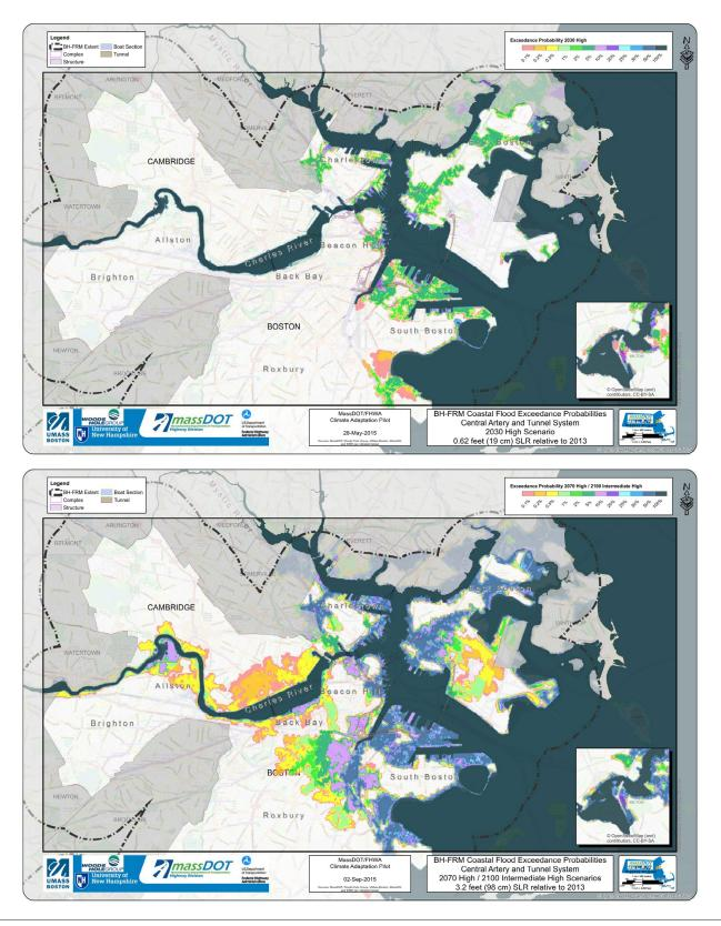
Figure 3.1: Coastal Flood Exceedance Maps from the 2015 FHWA Pilot Project with top showing projected inundation by 2030 (0.62 feet of SLR) and bottom showing projected inundation by 2070 (3.2 feet of SLR). (Source 2015 FHWA Pilot Project.)
