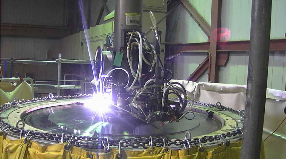
Welding the Lid on MPC #2
