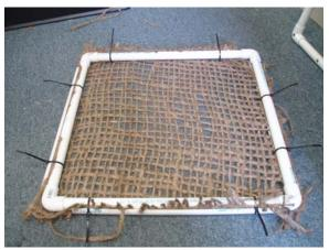
**Figure 4.** A PVC frame/jute mesh structure was constructed as a lighter-weight alternative to  $TERFs^{TM}$ .
