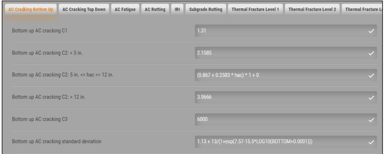
**Figure 37. Screen Shot of the PMED Software Displaying the Global Bottom-Up Fatigue Cracking Global Calibration Coefficients.**
