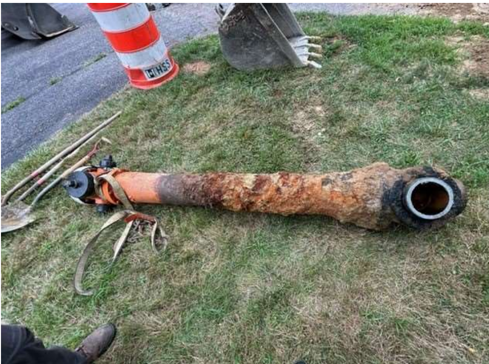
Photo 3: An old hydrant removed from service in Hanover. Hanover Water Department has a detailed hydrant mapping system and maintenance program to ensure that their hydrants are operable in advance of fire emergencies.
