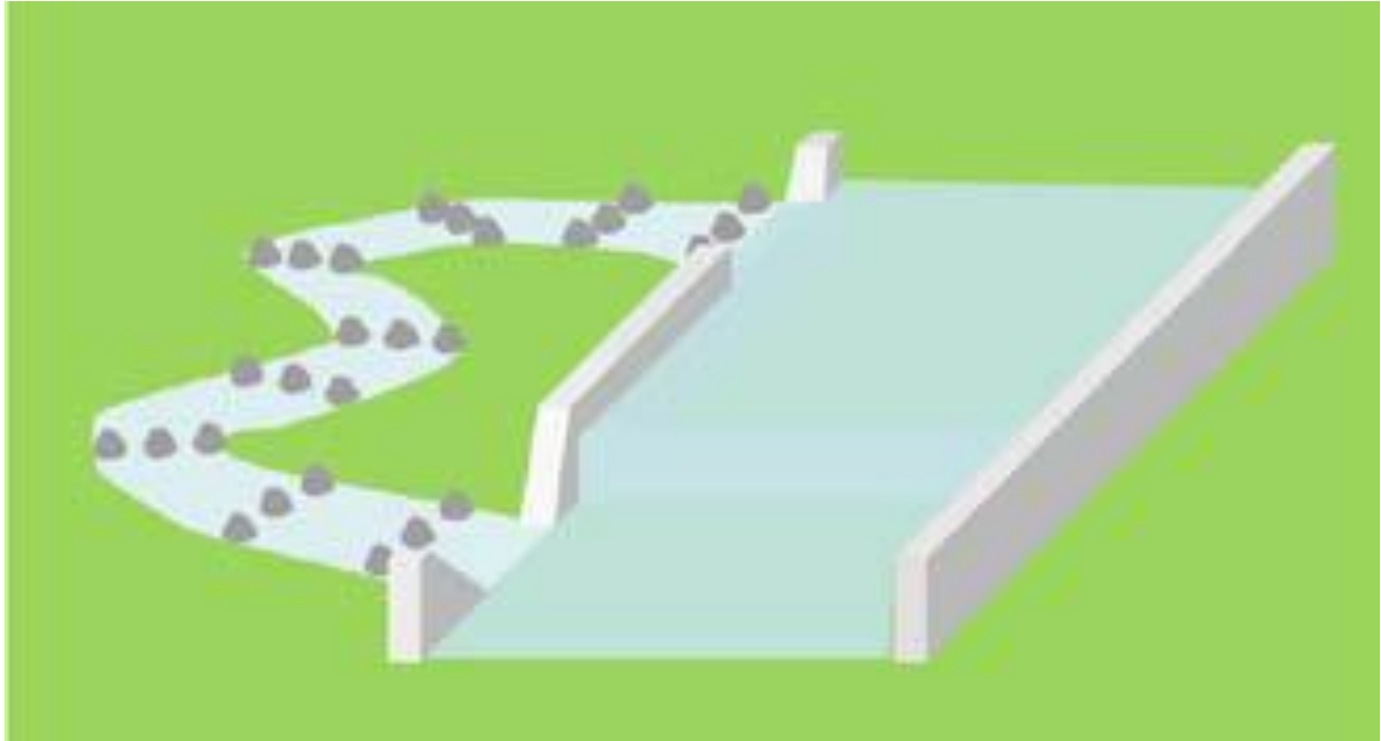
Nature-like fishway; bypass design
