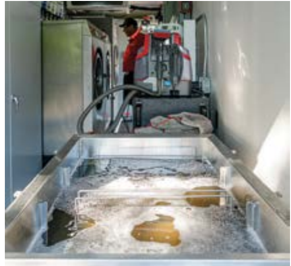
The ultrasonic cleaning unit is designed specifically for PPE. It processes helmets and boots and meets NFPA requirements.
