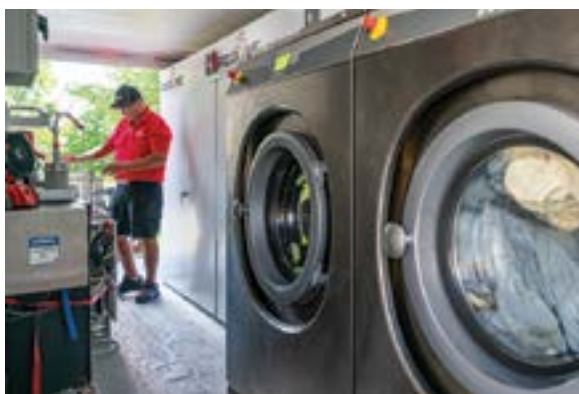
Foreground: Inner and outer shell gear extractors decontaminate the shells of PPE without breaking down sensitive materials. Background: Outer shell drying units allow controlled ventilation for careful drying of sensitive items including uniforms, helmets, and boots.
