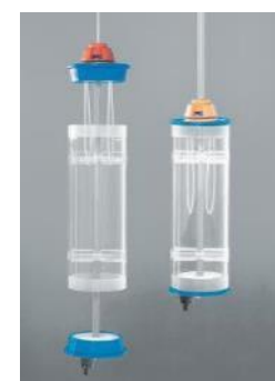
Kemmerer depth sampler
