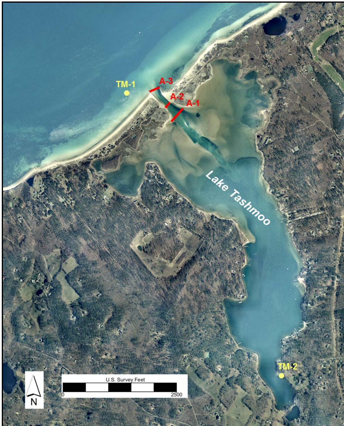
Figure V-2. Map of the study region identifying locations of the tide gauges used to measure water level variations throughout the system and locations of the ADCP transects (A 1-3). Two gauges were deployed for the 34-day period between July 19 and August 23, 2004. Each yellow dot represents the approximate locations of the tide gauges: (TM-1) Vineyard Sound (Offshore) and (TM-2) in Lake Tashmoo south of Brown Point. Each red line represents the location of an ADCP transect that was run hourly on August 11, 2004: (A-1) inside the inlet to Lake Tashmoo, (A-2) inside the inlet to Lake Tashmoo, and (A-3) located outside the mouth of the inlet to Lake Tashmoo
