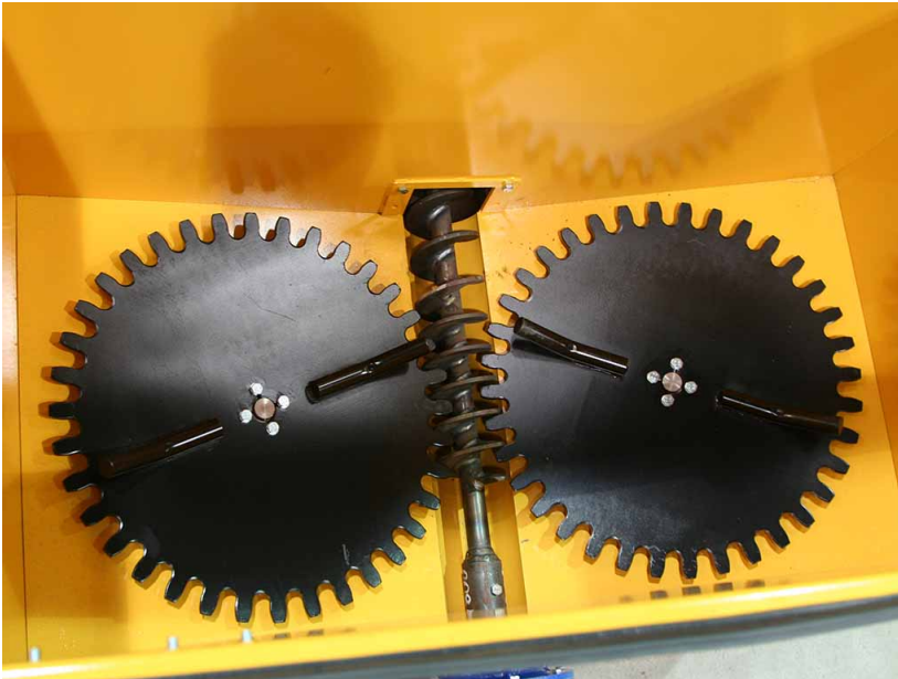
Figure 3 – Agitators on the bottom of the hopper (picture from manufacturer)
