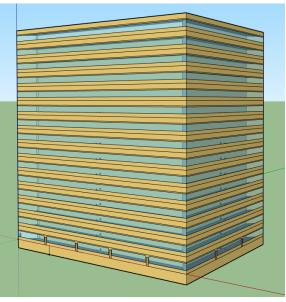
Heating system and an Electric-Heating alternative system along with envelope system improvements. The Office highrise geometry includes **614,400 gross sf** in four (15) stories above grade and 1 floor basement levels. Additional 38,357 sf. of penthouse space houses mechanical equipment. The building is slab below grade.
