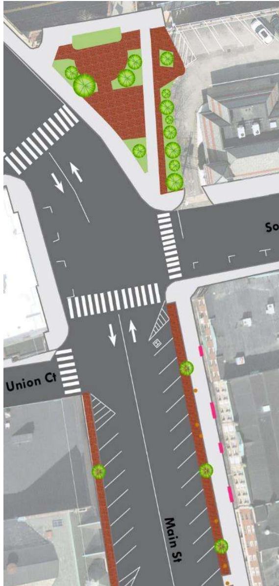
Layout pLan of before and after conditions for traffic calming and in-street outdoor dining on Main Street
