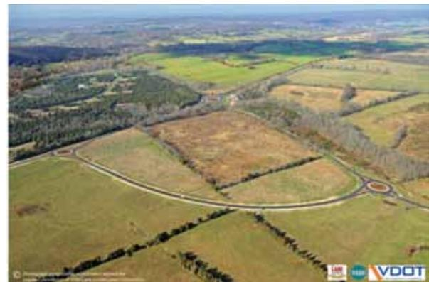
Along VA Route 50, the Gilberts Corner roundabout plan accommodates substantial turning movements between Route 50 and Route 15 by adding a new diagonal connecting road with additional roundabouts.
