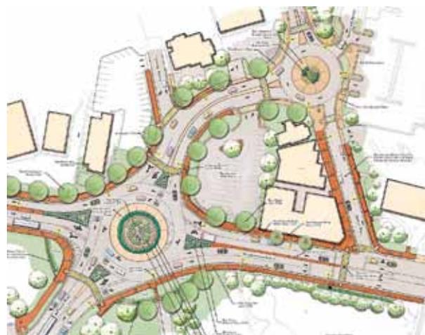
The roundabouts at the Hillsborough/Pullen (lower left) and Oberlin/Pullen (upper right) intersections reflect the variety of design options available in just this one type of intersection. Higher-volume, multi-lane roadways can still be accommodated with roundabouts through the use of two lanes in the circulating roadway.
