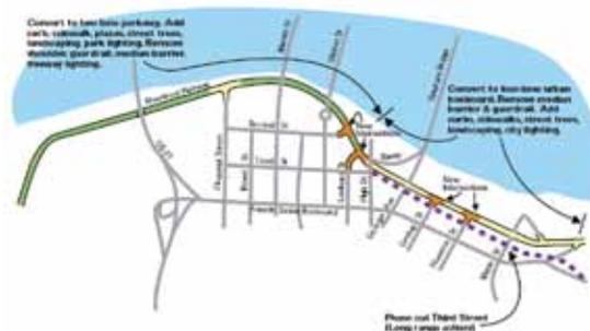
Recommended changes to Riverfront Parkway included the addition of access to downtown Chattanooga through new at-grade intersections and, in some places, the reduction of roadway width from four to two lanes. Designers made a case that the use of network preserved overall system capacity but that the re-design of the Parkway restored riverfront access from downtown.
