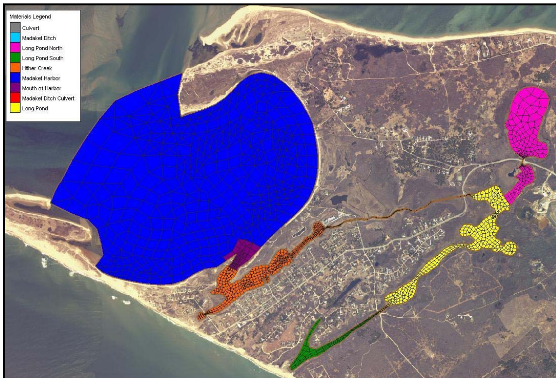
Figure V-8. The model finite element mesh developed for Madaket Harbor estuary system. The model seaward boundary was specified with a forcing function consisting of water elevation measurements obtained at the F Street Gage (S-1).
