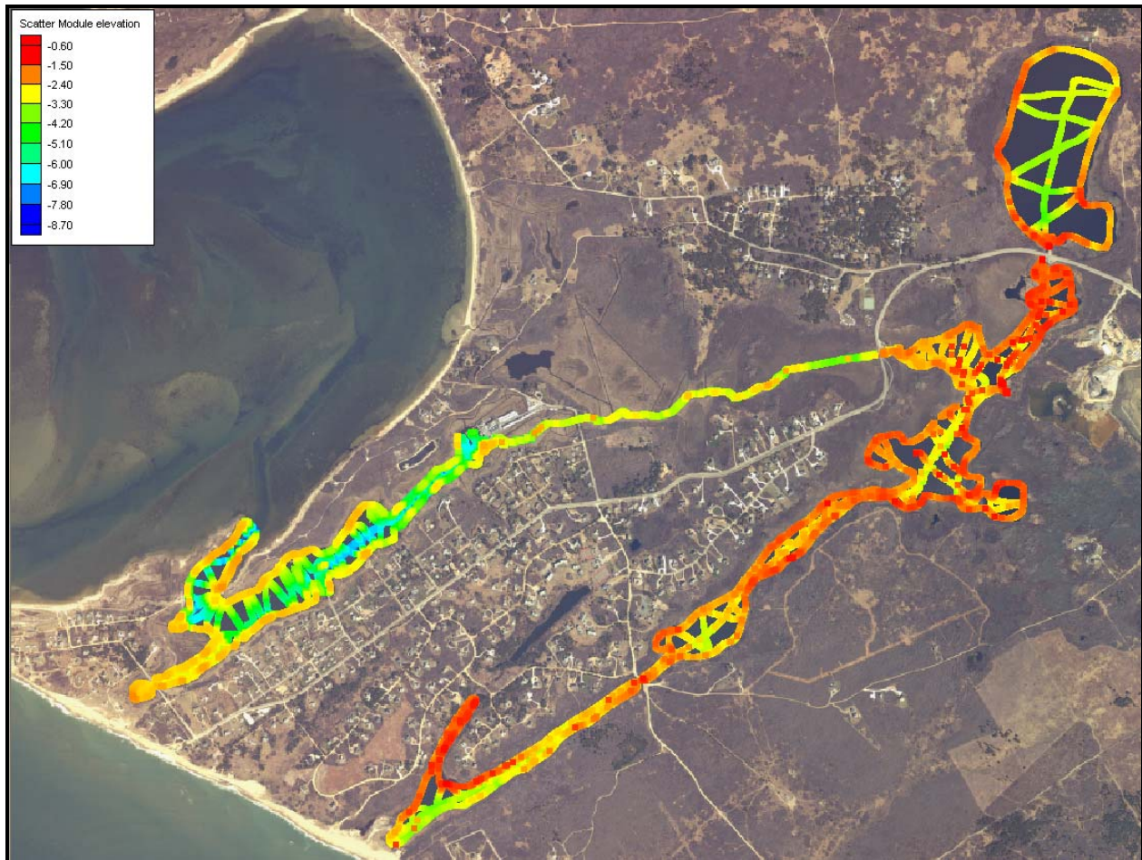
Figure V-3. Bathymetric data interpolated to the finite element mesh of hydrodynamic model.
