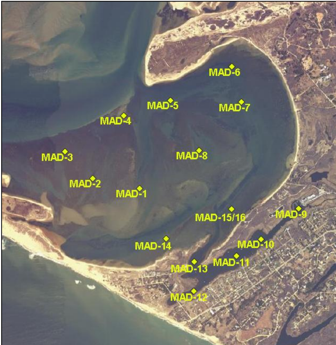
Figure IV-9. Madaket Harbor System (inclusive of Hither Creek) locations (yellow diamonds) of sediment sample collection for determination of nitrogen regeneration rates. Numbers are for reference in Table IV-3.
