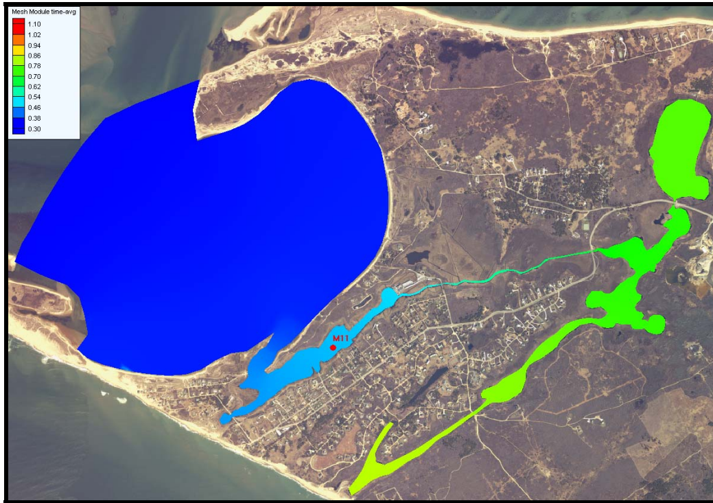
Figure VIII-1. Contour plot of modeled total nitrogen concentrations (mg/L) in the Madaket Harbor estuary, for threshold conditions. Threshold station is shown (0.45 mg/L at M11 in Hither Creek).
