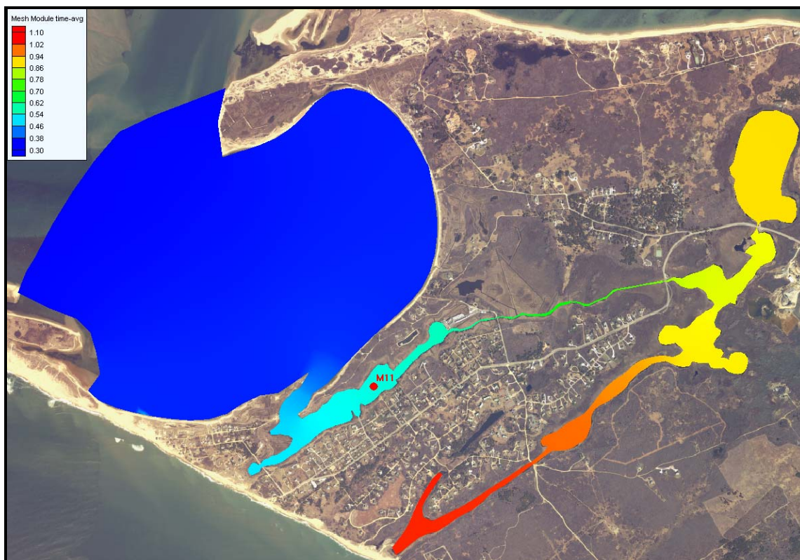
Figure VI-7. Contour plots of modeled total nitrogen concentrations (mg/L) in Madaket Harbor System, for projected build-out loading conditions, and bathymetry. The approximate location of the sentinel threshold station for Madaket Harbor System (M11) is shown.
