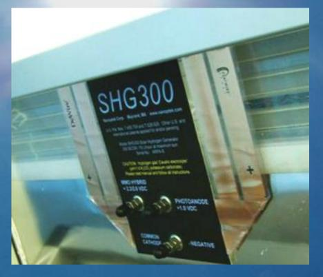
MMO anode behind photoanode can use renewable electricity to continue producing H2 without sun: conventional electrolysis MMO and photoanodes can operate simultaneously Greatly improves ROI and cost per kg SHG 300 as buffer between intermittant renewables (solar and wind) and, with fuel cell, on-demand power that utilities require Adds value to both sides of equation
