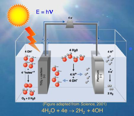
Basically an alkaline electrolyzer in which the anode is replaced with a photoanode The photoanode is Grade 1 titanium onto which a titanium dioxide (TiO<sub>2</sub>) photocatalytic semiconductor layer is grown by thermal oxidation
