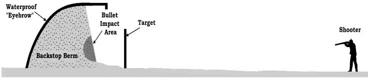
Side view of a rifle/pistol range backstop. An "eyebrow" prevents precipitation from eroding the backstop and helps to contain ricochets. Figure adapted from *Environmental Aspects of Construction and Management of Outdoor Shooting Ranges*, National Shooting Sports Foundation, 1997.
