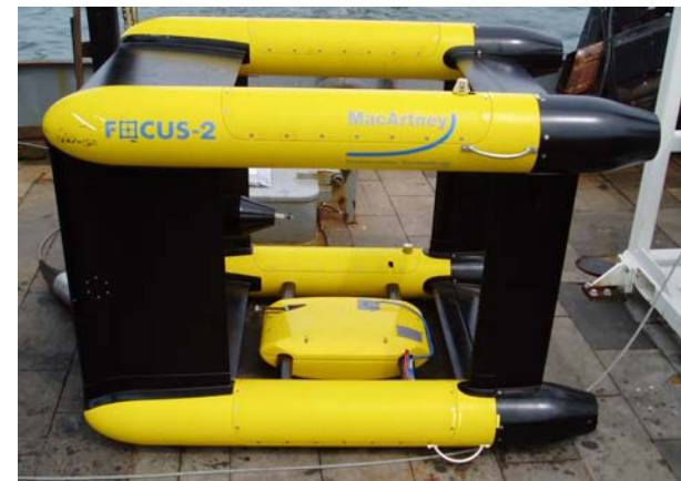
The towed underwater vehicle Focus-2, equipped with the Kongsberg EM3002 sonar head, sits on deck of the R/V Gloria Michelle during the second sea acceptance trial in June 2006.
