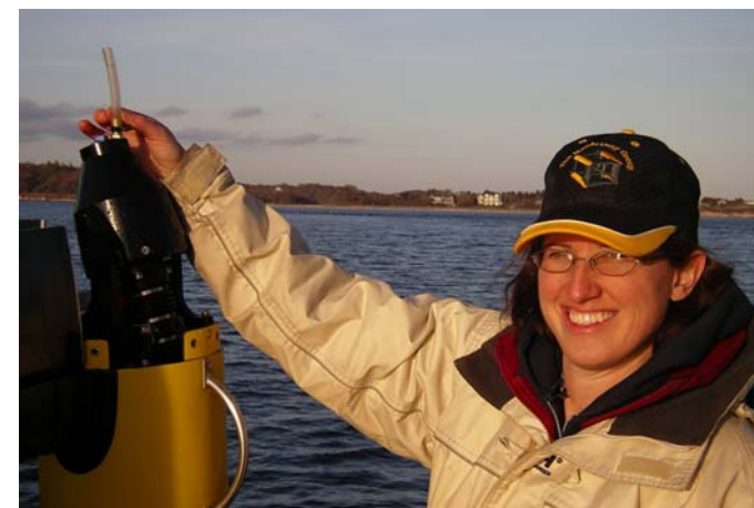
Dr. Kathryn Ford checks the silicon lubricant level of one of the motors of the towed underwater vehicle Focus-2 after a dive during the first sea acceptance trial in March of 2006.
