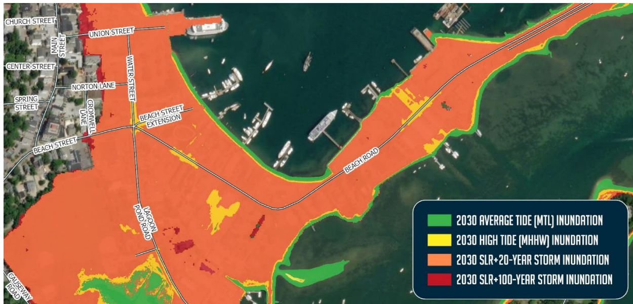
Figure 5 | Extent of Flooding in Vineyard Haven under Several Future Conditions
