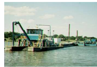
Hydraulic dredging: large cutterhead barge
