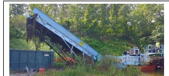
Mechanical harvester offloading to conveyor with transfer to rollaway hopper
