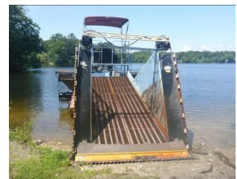
Cutting end of a mechanical harvester (above) and loaded hopper after harvest (below)
