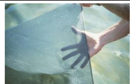
Porous weave benthic barrier (Aquascreen)
