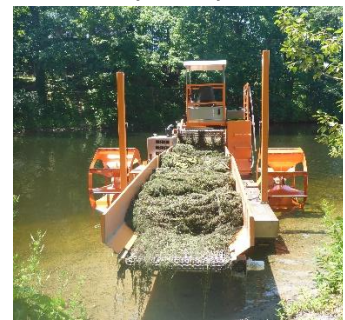
Cutting end of a mechanical harvester (above) and loaded hopper after harvest (below)
