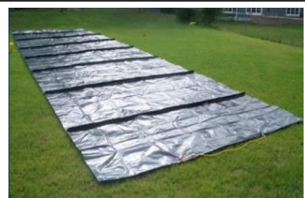
Non-porous benthic barrier with sleeves for rebar weights (LakeBottomBlanket) (Courtesy of Paul Grosjean)
