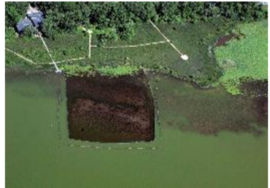
Carp enclosure area showing much clearer water in Lake Wingra, WI (photo by M. DeVries, courtesy of NALMS)
