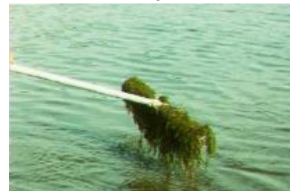
Commercially manufactured lake rake used to clear swim area of plants
