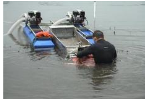
DASH: Diver puts plants into the suction tube (above) and plants are bagged at the surface (below)
