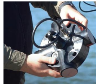
WaterIQTech (above) and buoy-mounted LG Sonic (below) sonicators (courtesy of WaterIQTech and LG Sonics)
