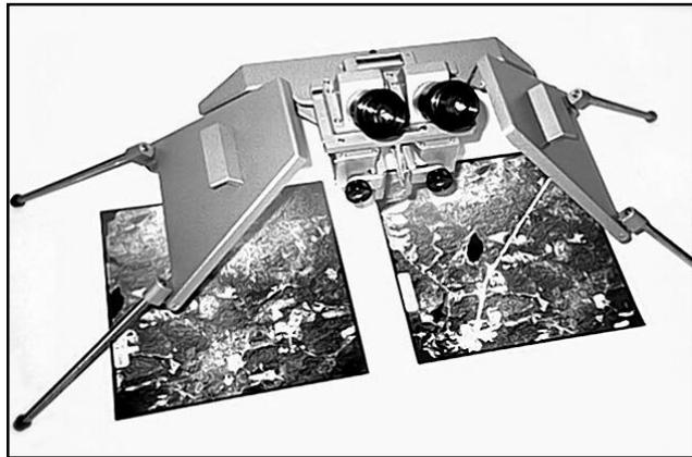
**Figure 2:** Mirror stereoscope
