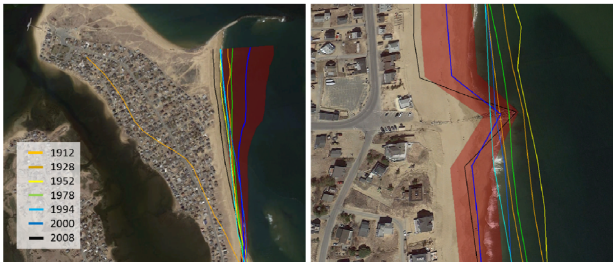
Figure 16. Examples from Plum Island illustrating the effect of anthropogenic influences on the shoreline position and uncertainty forecasts. On the left, the construction of a jetty changed the trajectory of the shoreline after 1912, but large uncertainty still exists in how the coast will evolve. On the right, the construction of a groins identified in the Kalman filter prediction.
