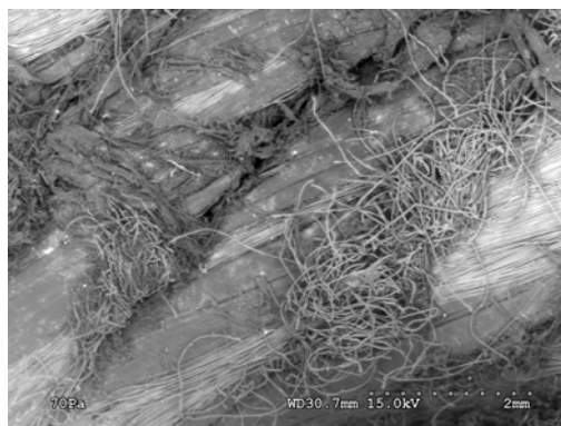
Figure 11. Outer face of sinking groundline, seen with Scanning Electron Microscope (TTI image)
