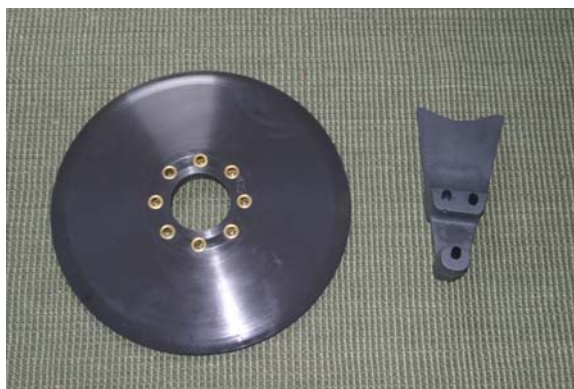
Figure 16. Polyurethane sheave liner and polyurethane knife made by Corrosion Control Resources.
