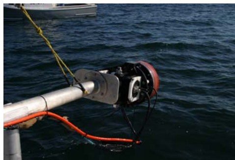
Figure 17. Multi beam transducer on adjustable arm
