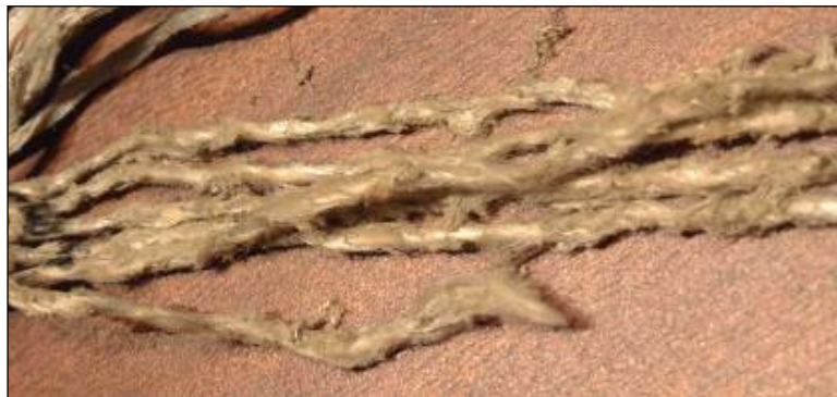
Figure 10. View of outer rope yarns from machine tested rope, showing external damage (TTI image).
