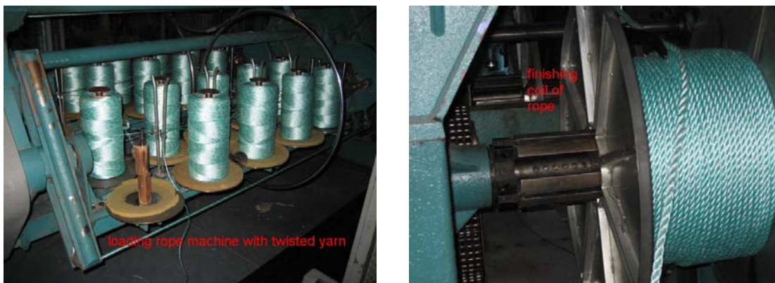
Figure 14. Fabrication process for Anacko sinking groundline made to TTI specifications.
