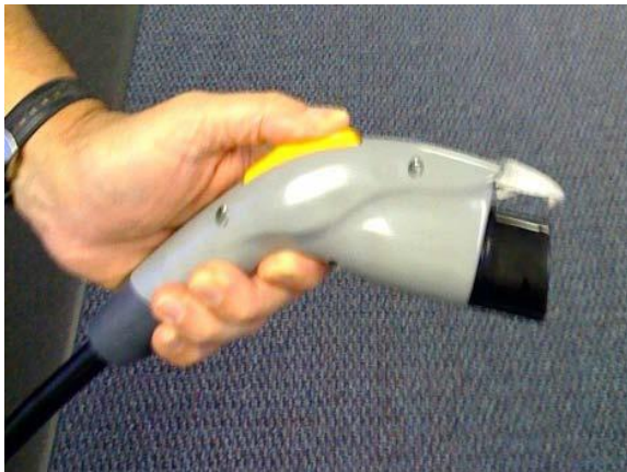
Figure 3: The J1772 Connector.
