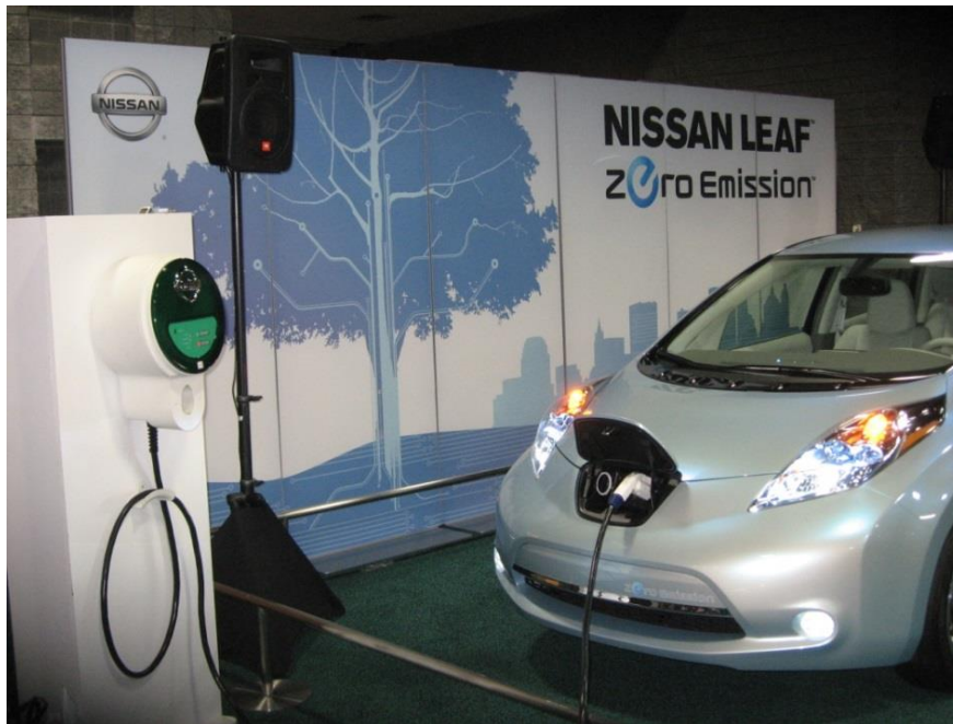
Figure 5: A Nissan Leaf using Level 2 charging.
