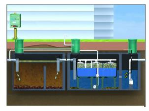
**Figure 4.17.** Enhanced I/A septic system. Graphic: SeptiTech/BioMicrobics ®.
