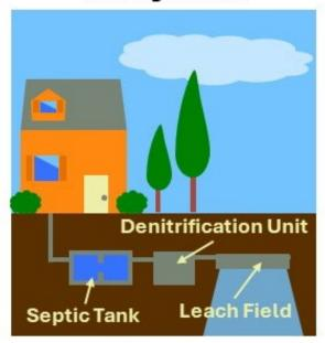
**Figure 4.16.** Comparison of a traditional septic system and an innovative/alternative. Not drawn to scale.
