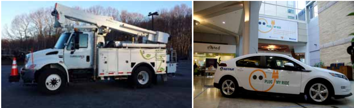
Figure 19. Eversource plug-in hybrid electric bucket truck and PEV.
