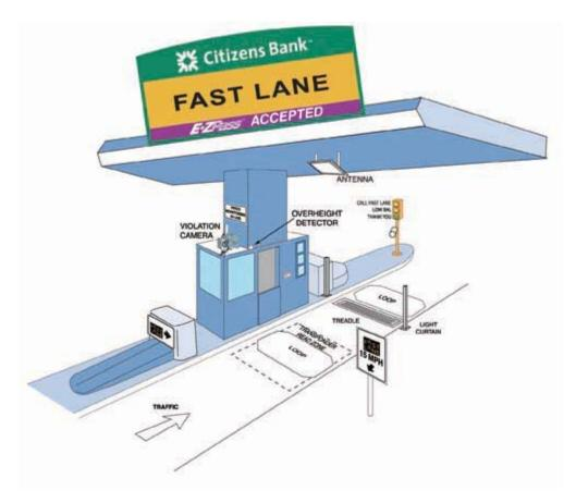
A Fast Lane-equipped vehicle travels through a Fast Lane at a toll plaza. The transponder identifies the vehicle as a participant in the program and gives the vehicle a green light, indicating that the transponder has automatically recorded the toll to the member's Fast Lane account.
